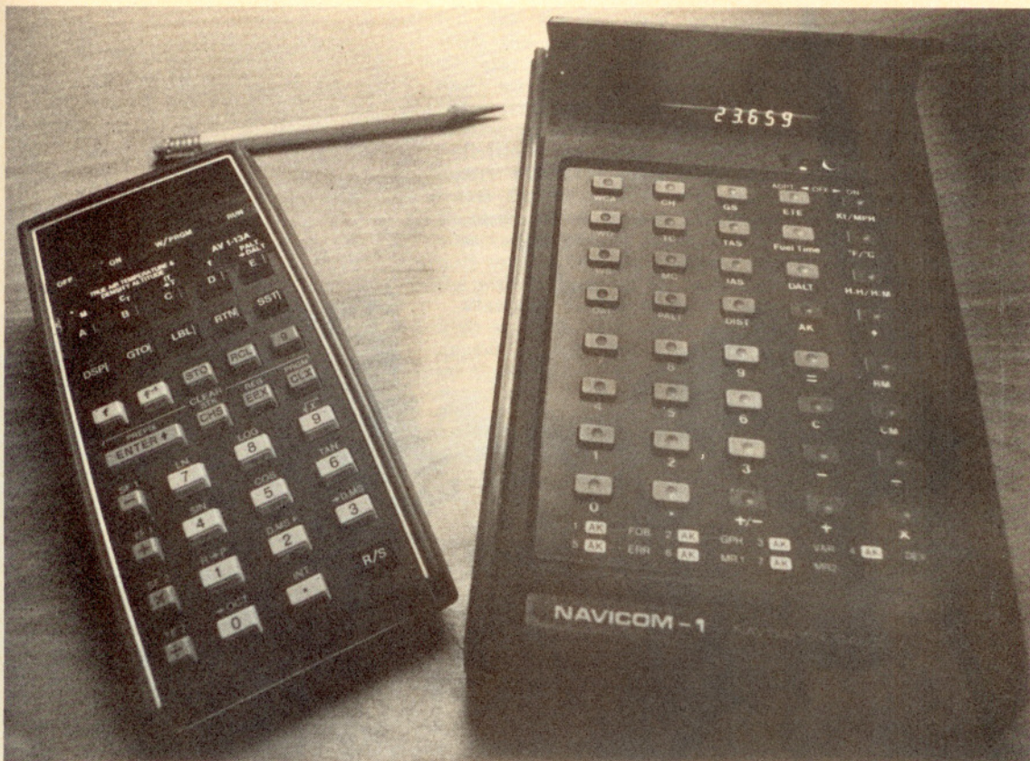
Hewlett-Packard's HP-65, left, will perform an unending variety of computations, while the Systek Corp.'s Navcom-1, right, is more of an electronic E6B.
